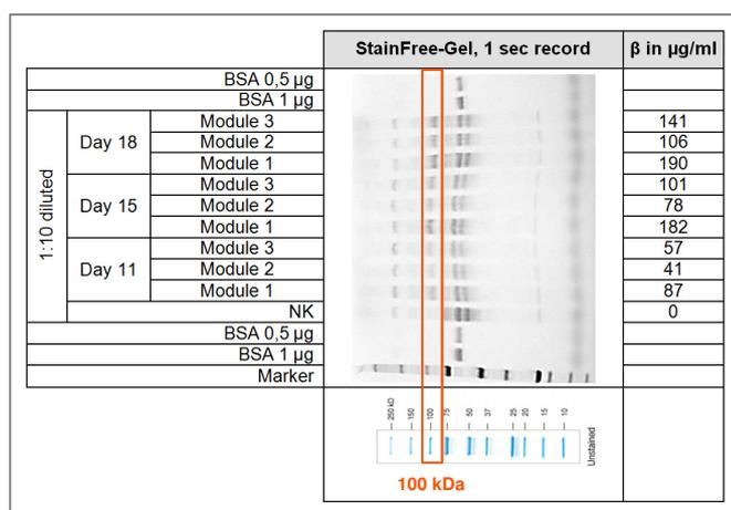
Fig.3: StainFree-Gel, applied are cell culture supernatants from the ECS of the 3 bioreactors on day 11, 15 and 18 and the protein concentration measured in  $\mu\text{g/ml}$
