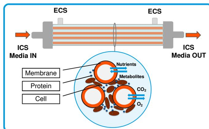
Fig. 1: Scheme of a cross section through a hollow fiber module and cultivation of cells in the ECS
