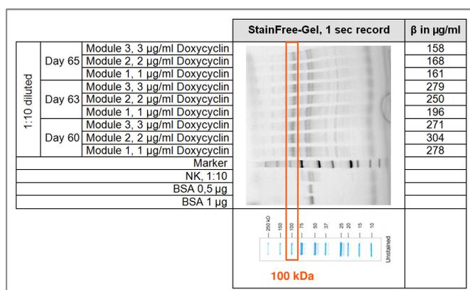
Fig.5: StainFree-Gel, applied are cell culture supernatants from the ECS of the 3 bioreactors on day 60, 63 and 65 and the protein concentration measured in  $\mu\text{g/ml}$  with adjusted concentrations of the induction antibiotic Doxycyclin in the ICS and ECS medium
