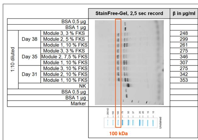
Fig.4: StainFree-Gel, applied are cell culture supernatants from the ECS of the 3 bioreactors on day 31, 35 and 38 and the protein concentration measured in  $\mu\text{g/ml}$  under reduced FCS concentration in the ECS medium
